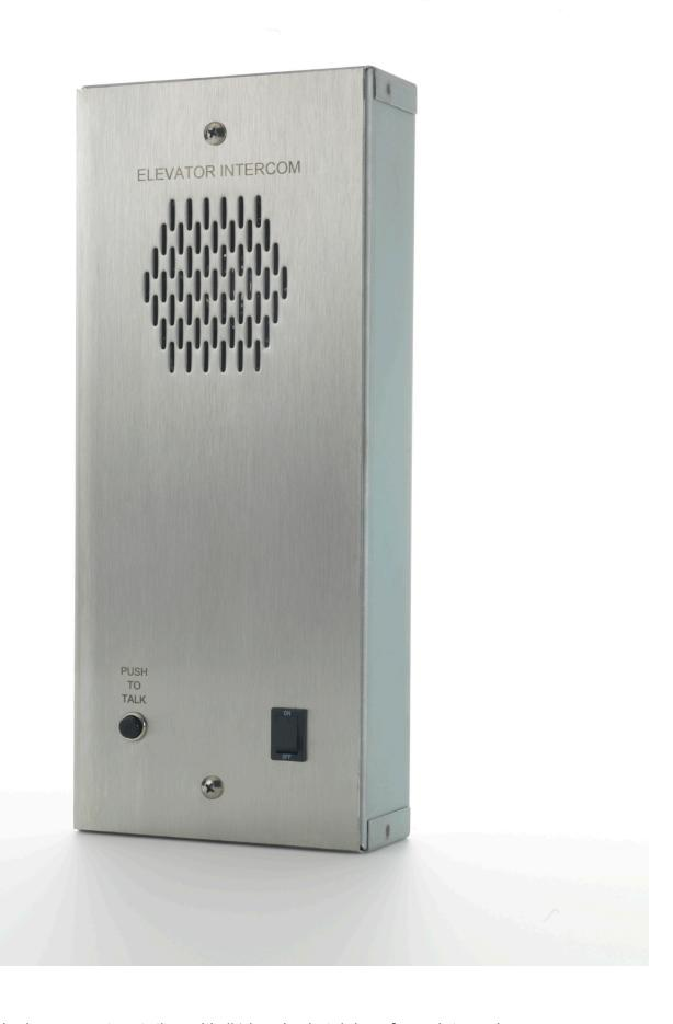
Everclear  $^{\circ}$ 0 intercom – Single car master station with #4 brushed stainless face plate and corrosion resistant EG steel enclosures for machine room surface mounting. Size 5-1/8" x 12-1/8" x 1-15/16" deep.
