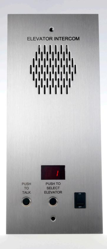
Everclear ® intercom with #4 brushed stainless finish, low-profile vandal resistant controls and 7-segment LED display. Size 5" x 12". Standard EG steel corrosion resistant enclosures are flush mount (recessed) for lobby and surface mount for machine rooms (Multicar shown)
