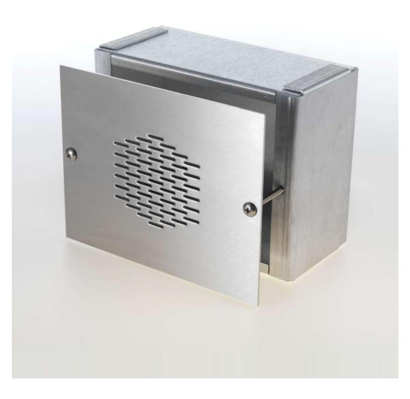
Everclear @ intercom optional car ceiling enclosure facilitates installing the car amplifier either above or below the car ceiling. Aluminum enclosure with #4 brushed stainless face plate. Size 6-1/2° x 5-3/16° x 3° deep.
